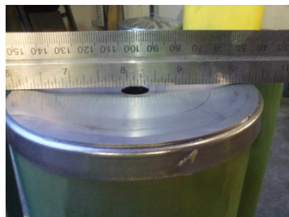
Over-Torqued Example From The Field
